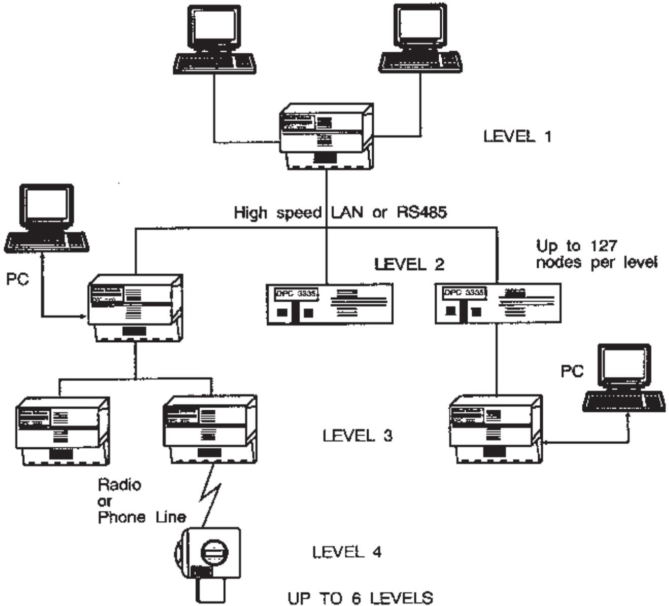
This hierarchy can extend up to six levels deep. Each intermediate node has both master and slave capability through separate communication ports. This architecture lends itself very well to the typical geographical distribution of controllers in most SCADA system applications. It also allows multiple asynchronous communications to occur throughout the network since each network branch can communicate simultaneously.
